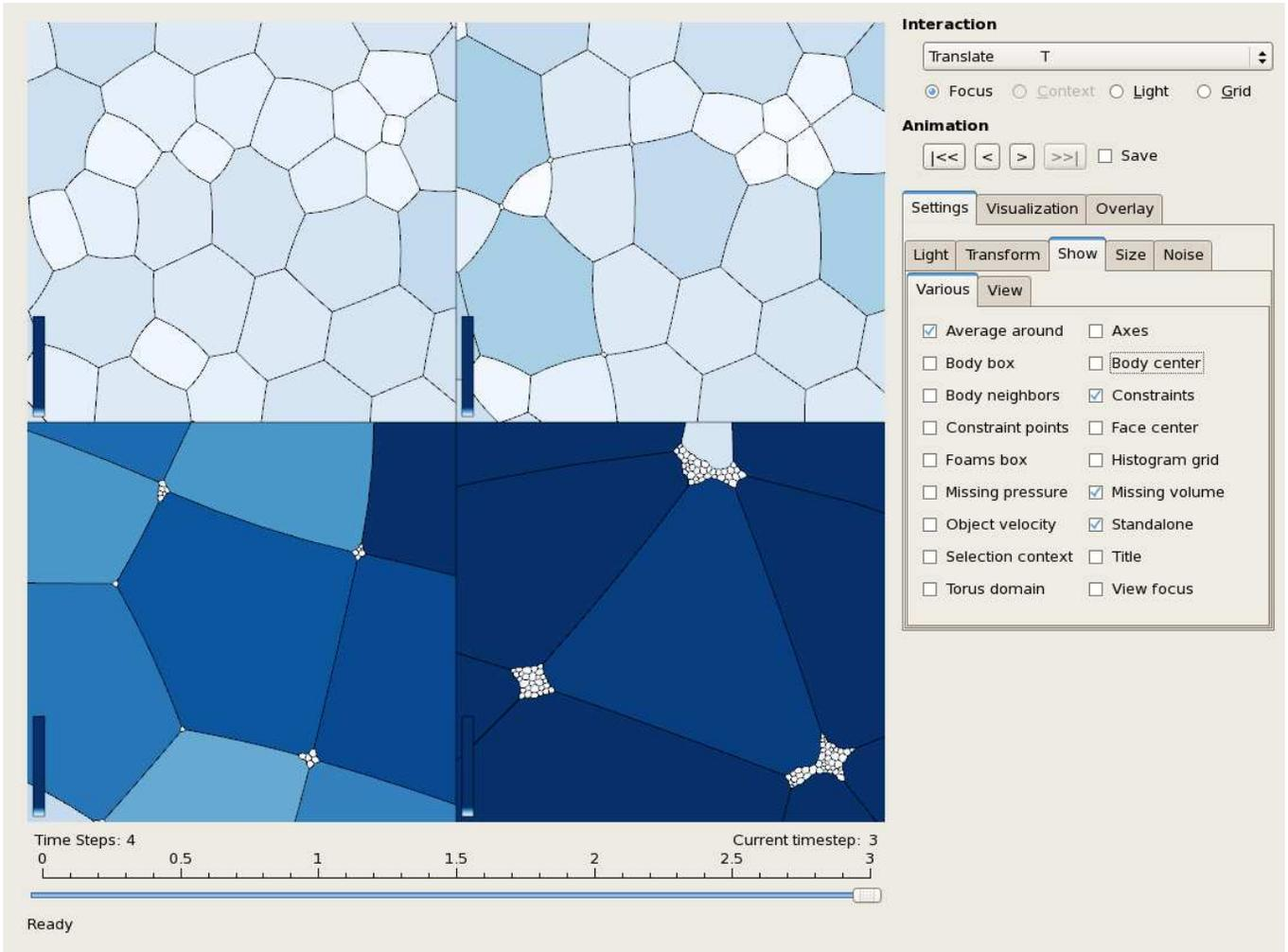
Figure 1: A screenshot of FoamVis for a simulation in which a foam containing a mixture of two gases undergoes diffusion-driven coarsening. The foam is shown at timesteps  $10^2$ ,  $10^3$ ,  $10^4$  and  $10^5$ . Bubbles are coloured by area, and the same bubble is kept at the centre of the field of view. The foam gradually segregates into a few large bubbles with equal pressure, with many smaller bubbles of roughly equal size clustered around their vertices.
