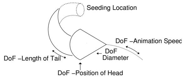
Figure 5: The streamcomet promotes four interactive degrees of freedom: (1) the position of the comet head along the path of integration, (2) the diameter of the comet head and tail, (3) the length of the comet tail, and optionally (4) the animation speed of the comets
