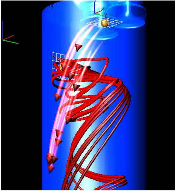
Figure 6: Two seeding planes in the combustion chamber of a piston valve: one seeding streamcomets, the other seeding shaded streamlines.
