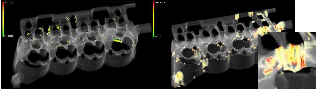
Fig. 6 (left) Areas of temperature t \geq 363^\circ K are interactively-specified by the user and rendered in focus. (right) The regions of very high pressure gradient, (inset) an unexpected high pressure gradient.
