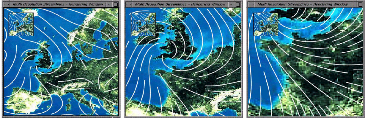
Figure 8: Three images from an interactive exploration of a vector field using the MR viewer 34 . A suitable level of resolution can be chosen while maintaining a roughly constant stream-line density.
