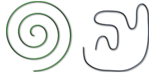
Fig. 2. Both of these curves exhibit very similar curvature magnitude values. Therefore, a single global measure fails to distinguish streamline sufficiently. In this case, the tortuosity attribute would fair better but there are cases where this would also fail. A better method creates a distinctive signature for the streamlines using density-based attributes.
