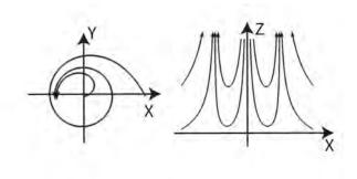
Fig. 6: The Sullivan Vortex viewed in the x-y plane (left) and the x-z plane (right).
