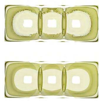
Fig. 3: This figure compares the neutral surface of the three ball simulation using the Marching Tetrahedra method (top) and the A-patches method (bottom). Notice that not only does the A-patches method better preserves geometry details such as the outline of the holes, it also reduces the topological errors caused by the Marching Tetrahedra method.
