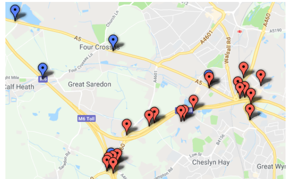
Fig. 4. Map showing dense (red markers) and sparse (blue markers) hot spots identified by our fuzzy HSID algorithm. Dense hot spots tend occur at road junction, while sparse hot spots occur on straighter stretches of road.
