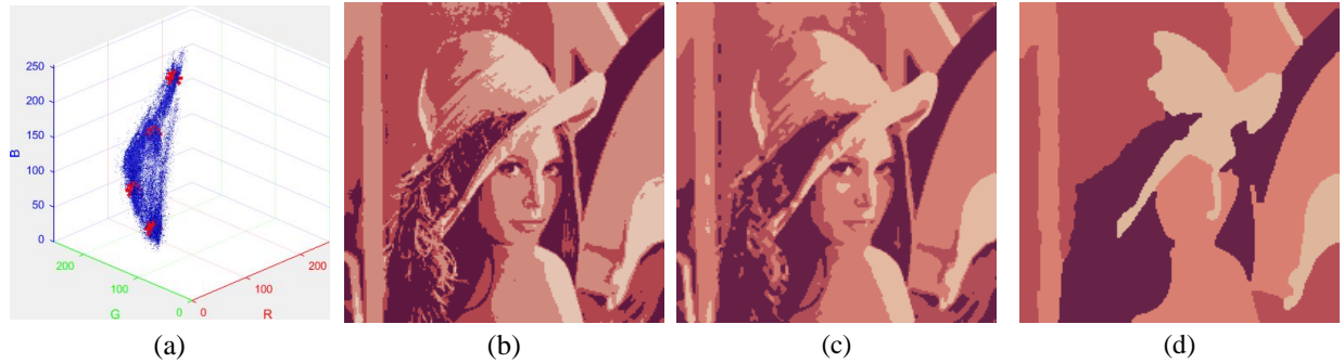
Figure 2. (a) RGB distribution and peak locations (b) segmented image by 3DHP, m=4 , (c) segmented image by FCM, m=4 , (d) segmented image by SFFCM, m=4
