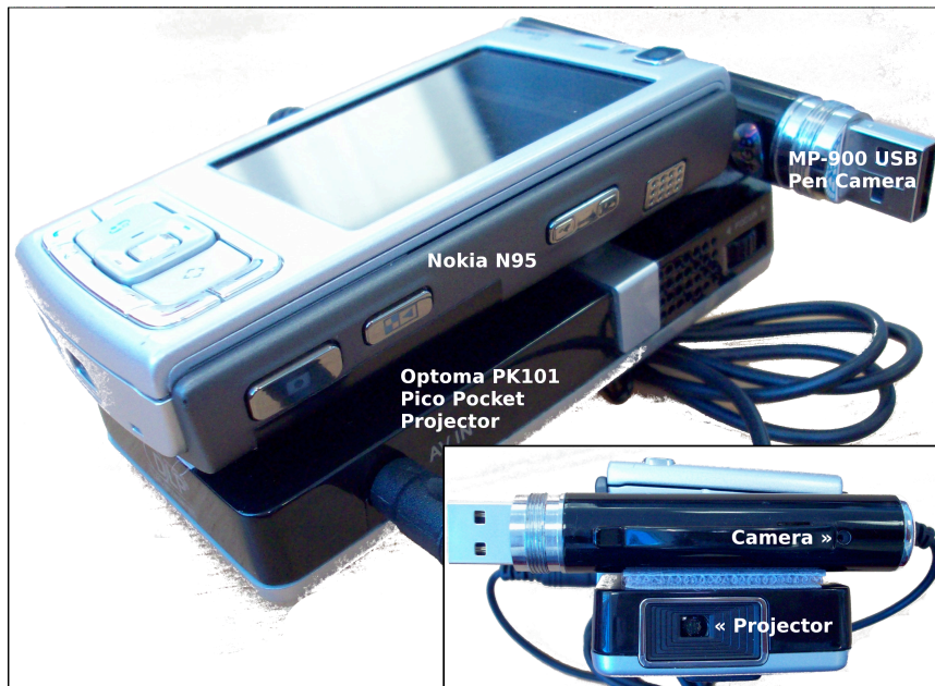
Fig. 1 Study 1 apparatus, where the projector and a pen video camera face the same direction
