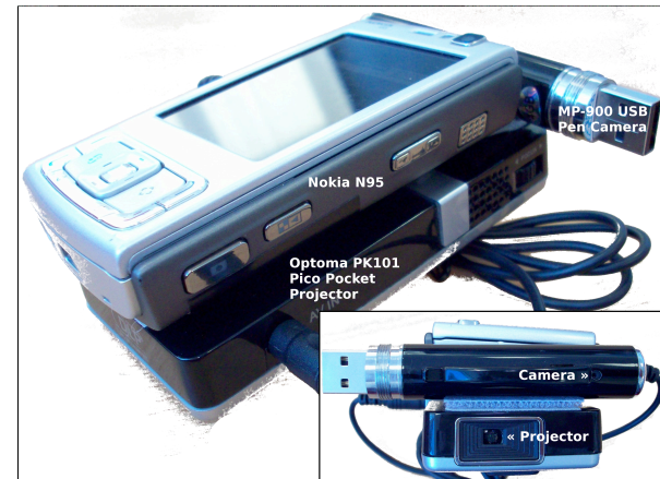
Figure 1: Prototype projector phone, where the projector and pen video camera face the same direction.
