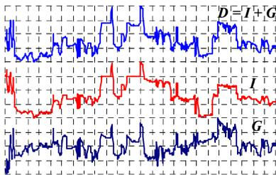
**Fig. 5.** A scan line from the images in Fig. 1, all three signals are scaled to 0 ~ 255. It is seen that the gain map image (bottom line) strictly follows the changes of the original image (middle line). The result image (top line) and the original image (middle line) have exactly the same edge directions. It is also seen that the sum image  $D$  (top line) has more local details than the logarithm of the original radiance map (middle line).
