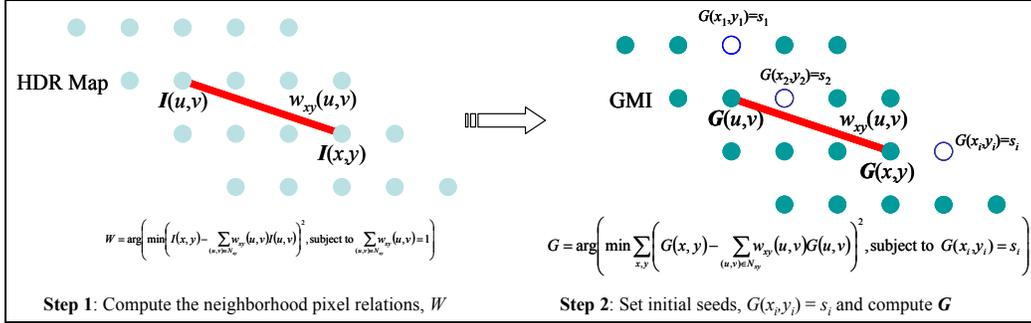
**Fig. 4:** Schematic of linear neighborhood embedding (LNE) and its application to computing the gain map image. The process has two steps. First, we compute the local neighborhood pixel relations by solving a quadratic optimization problem. Secondly, we seed some initial GMI pixels and use the neighborhood pixel relations computed from step 1 to compute the GMI by solving a constrained optimization problem.
