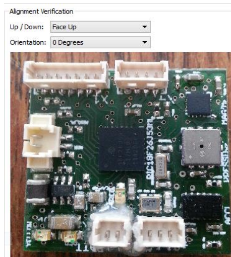
27 28 29 30 31 32 33 34 35 36 37 38 39 40 41 42 43 44 45 46 47 48 49 50 51 52 53 54 55 56 57 58 59 60 61 62 63 64 65 Figure 2 - This image shows the alignment correction step. An image of the sensor board is updated to show the alignment selected.
