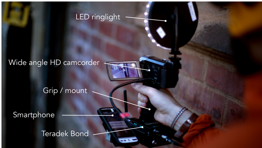
Figure 2: Runner camera rig (image credit: Blast Theory)
