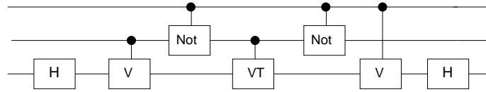
representing them cannot be separated into individual state vectors. This means that, despite the appearance to the contrary, it is not possible to operate on any of the lines individually. Instead the circuit defines a linear operation on the entire state:
