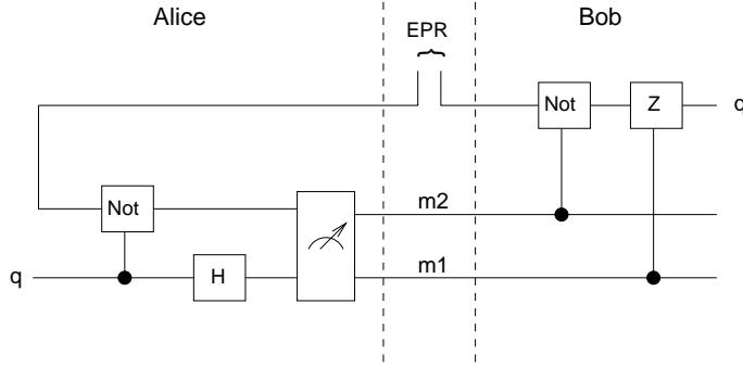
The calculation proceeds as follows. First Alice interacts with the unknown qubit  $q$  and her half of the *epr* state. Then Alice performs a measurement collapsing her quantum state and getting two classical bits  $m_1$  and  $m_2$  that she transmits to Bob using a classical channel of communication.
